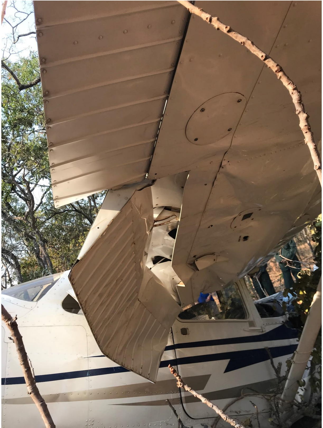
Fig. 4: Wings and Secondary Control Surface (Flap) Damaged, Detached Wing Tip and Punctured Fuel Tank
