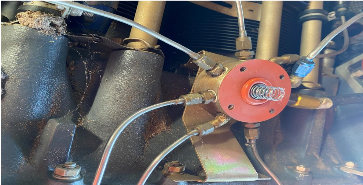
Fig.7: Fuel Flow divider and diaphragm intact
