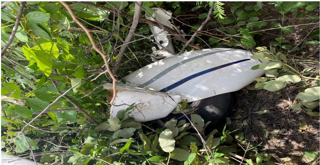
Fig.2: Right Hand Main Landing Gear Detached from the Wing
