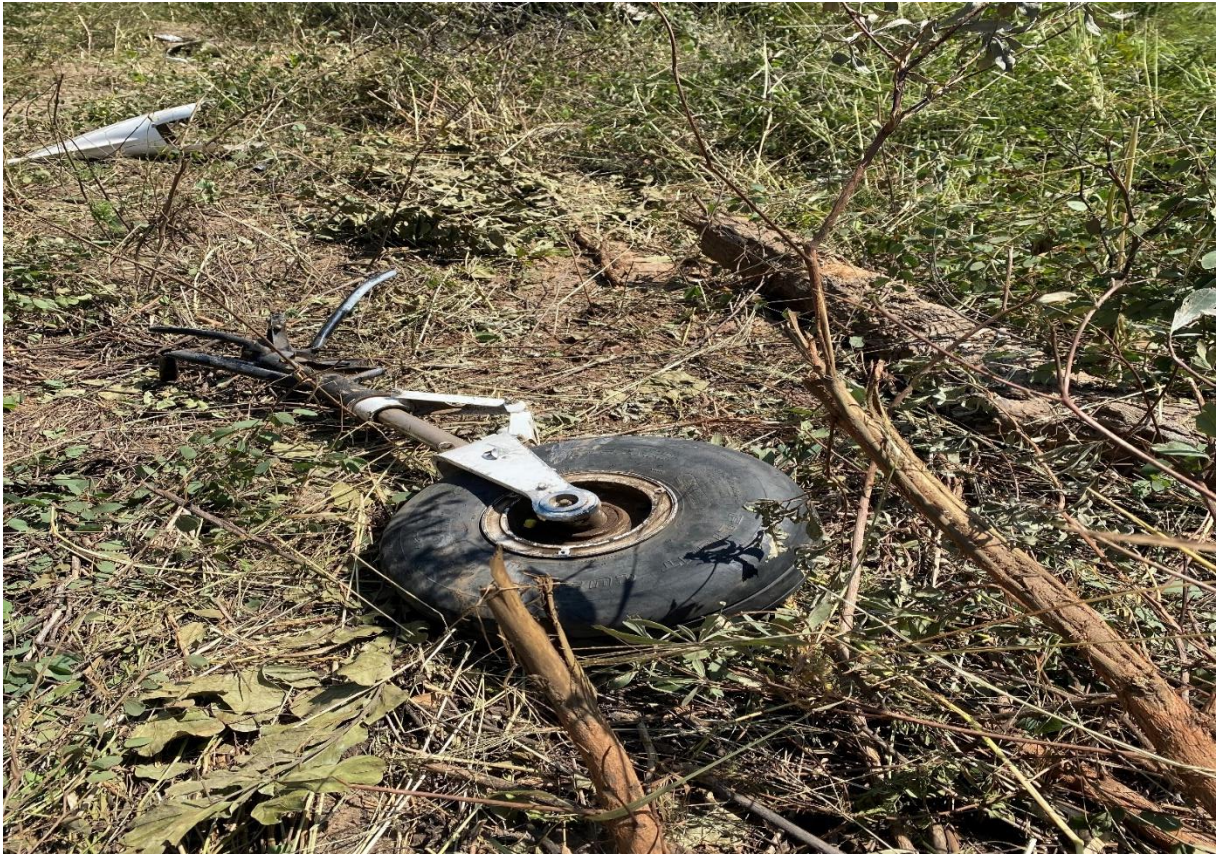
Fig.1: Nose Landing Gear Detached from the Airframe
