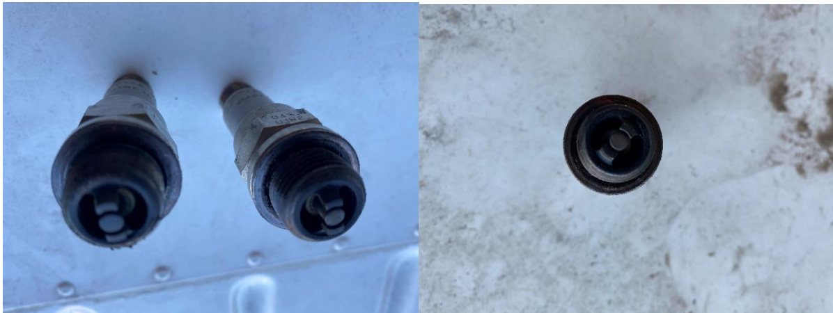
Fig.7: Fuel Flow divider and diaphragm intact
