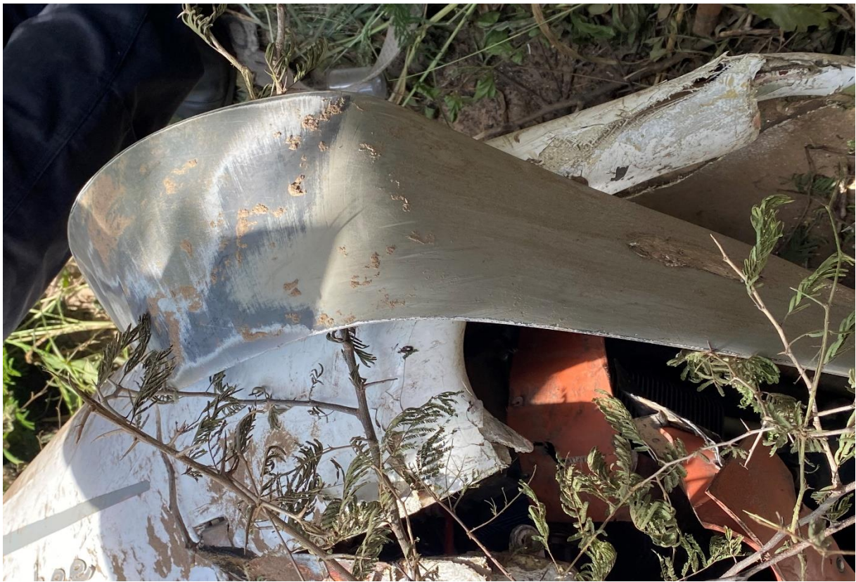
Fig.6: Propeller Blades Bent Backwards and Scratched at the Tip
