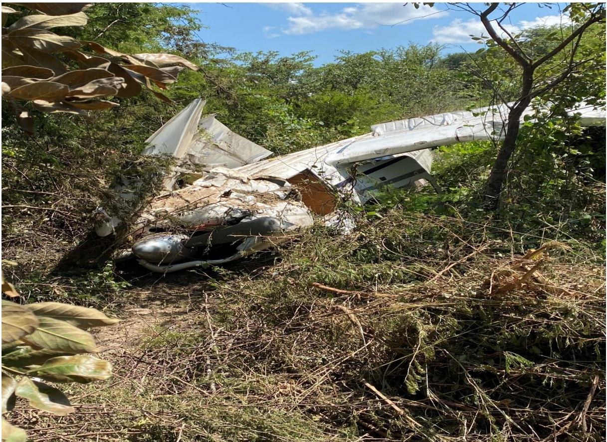
Fig 4: Left Wing Compressed, Folded in Several Sections and Partially Split at the Wing Root Area with Some Pieces of Frames Broken off and Spread.
