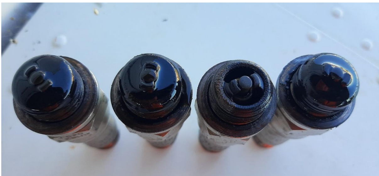
Fig.8: Some Spark Plugs Found with and without Oil
